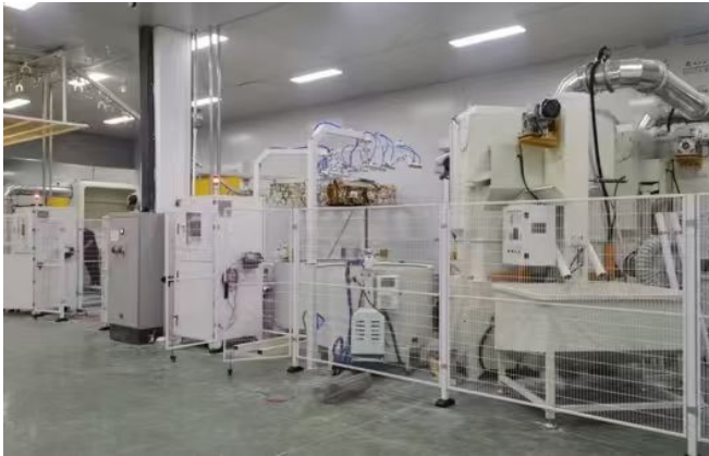
Robotic shell-building line
